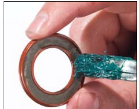
Figure 24. Greasing the bearing covers
